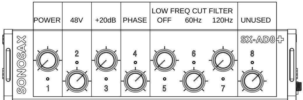
When input configuration is enabled, knobs and LEDs 1 to 7 are used to change input setup:
