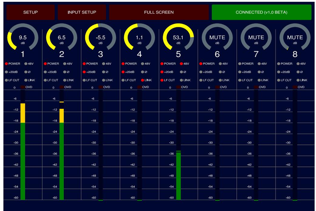
The main page consists of a top menu and 8 identical input slices.
