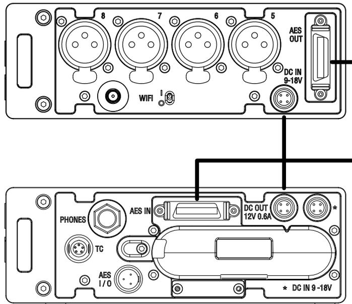
Don't forget to enable DC output in the SX-R4+ POWER menu. As soon as both devices are powered, the SX-AD8+ will connect with the SX-R4+. When operating in this mode:
